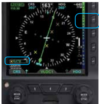
Figure 3-18 Lightning Overlay On Displaying WX-500 Strike Data
