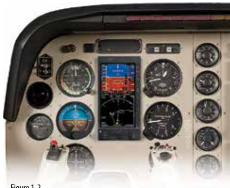
Figure 1-2 Single Display EFD1000 PFD System
