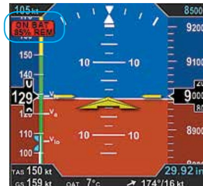
Figure 6-2 Battery Charge Remaining
