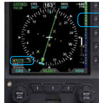
Figure 3-35 Lightning Overlay On Displaying WX-500 Strike Area
