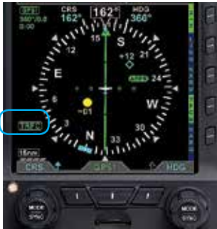
Figure 4-127 Traffic Overlay Enabled
