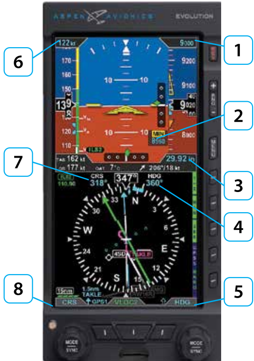
Figure 2-3 Left and Right Knobs and Corresponding Fields
