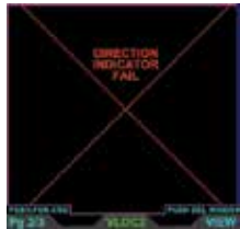
Figure 6-15 Direction Indicator Fail
