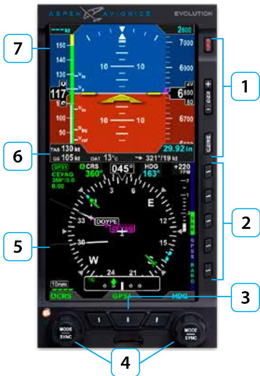
Figure 1 EFD1000 PFD Display, Knobs, Buttons, and Keys
