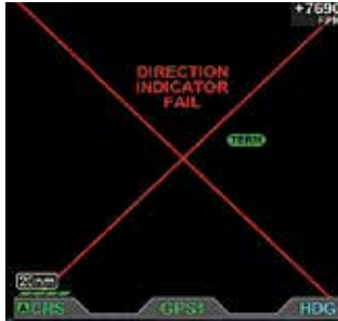
Figure 4-86 Direction Indicator Fail
