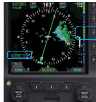
Figure 3-17 Data Link Weather Overlay On
